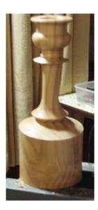
Turning commenced by rounding off the raw blank between centres and turning a tenon at one end to suit the chuck. Once in the chuck, and retaining a measure of support from the tailstock, one end of the blank was selected as the base and left in the round. The cup and a collar detail below were turned at the other end. A Forstner bit was used to drill out the hole for the candle holder.
