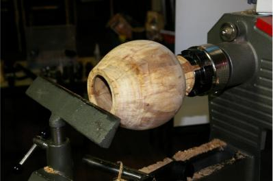
The base of the vessel is left thick at this stage to provide additional support during the hollowing phase. Initial roughing out of the interior is followed by working down in 2" (50mm) steps taking the thickness down to just over 1/8 inch (4mm). Remember that all this work is being done in an end grain piece. Tracy switched to a tear drop scraper for the final finishing of the interior.
