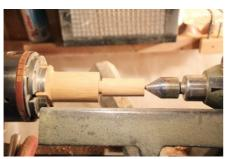
Begin to round over the 'head' section of the bird with gauge or skew (!) also reducing the area between body and head a little more but leaving enough strength in the wood for the next stage.
