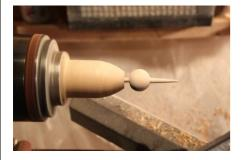
Reduce the end nearest the tailstock to 25mm diameter and then measure 35mm back from the tailstock end to define the beak (which should leave 25mm remaining for the head). Reduce this end
