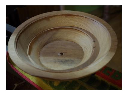
The glued assembly was remounted on the lathe using the same screw chuck and hole that had been employed in the initial turning of the rings. This hole was on what had now become the upper face of the base ring and the bowl was therefore mounted with its open face towards the headstock, in the correct position for the outside of it to be turned and finished.
