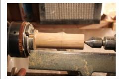
Reduce the square stock to a cylinder and mark off 60mm from the tailstock end to define the head and beak. Part in to the left of this line to a diameter of approx 20mm.
