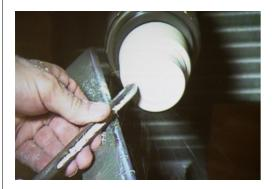
Shaping of the back of the head and refinement of the overall shape continued until such time as the back was finally parted through.
