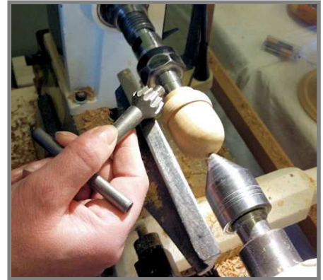
Dawn discovered that if necessary a chuck key can be used as a texturing tool for the cup of an acorn!
