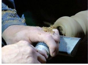
A jam chuck was next prepared for finishing the underside of the finial. This technique relies on the finial being small enough
