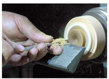
Undercutting the rim with the Jason Breach skew.
