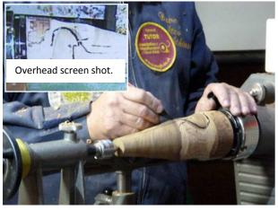
After roughing to a form, the cone approximate shape and size for finished box and finial were marked out as shown (left), allowing sufficient material for parting between finial and the box,
