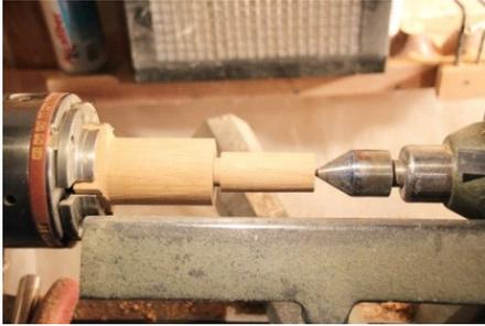
Begin to round over the 'head' section of the bird with gauge or skew (!) also reducing the area between body and head a little more but leaving enough strength in the wood for the next stage.
