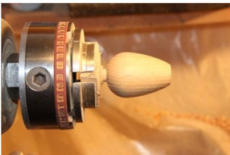
Part into the wood close to the chuck and turn the remaining wood to form an 'egg' shape where the widest portion is about 1/3<sup>rd</sup> of the length.
