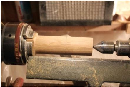
Reduce the square stock to a cylinder and mark off 60mm from the tailstock end to define the head and beak. Part in to the left of this line to a diameter of approx 20mm.
