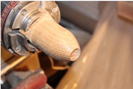
Hollow the end of the body so that the head can sit comfortably in the recess.
