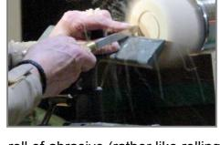
When sanding an "intermittent face", such as the on a winged bowl, it can be useful to make a sanding pad using wood shavings inside a
