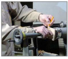
The piece was then reversed on the chuck and held on the recess, care being taken not to apply too much pressure which might split the wood. The tailstock was used to provide support to enable the top to be shaped using similar procedures to those used to shape the base but leaving the centre portion high to form a knob or spigot. This
