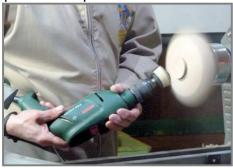
showing where the corners are. High rotation speed and sharp tools are the key to achieving good results and for this demo most of the turning was carried out at approximately 3000rpm. The shape of the bottom of the base was what Steve described as a "soft ogee", using a pull cut
