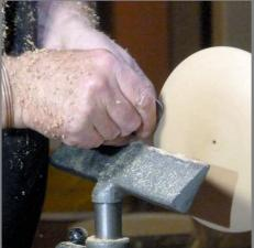
During the evening, Mark used only two turning tools; a small bowl gouge and a shear scraper, and did no sanding at all.
