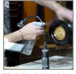
embers should cause an explosion. It is also important to make sure the lathe is clear of shavings and dust when performing the scorching. Mark laid a fire proof board on the lathe bed for added protection.
