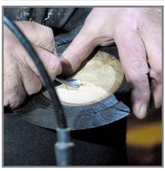
With the wood mounted on a screw chuck, Mark trued and faced it and proceeded to form a smooth curve to a very thin edge. A hand held cabinet scraper, used negative rake at 45° to the surface, was then used to give a fine finish. Then, using a gas blow torch, he the surface. scorched Mark explained that he uses "professional" torch that runs MAPP gas. This burns at a much higher
