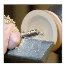
The final item was a "vase", again turned from a small piece of oak. After turning a shallow bowl, Mark cut this is half (along the grain) and joined glued the two halve together. A small flat was formed by sawing off a small section to allow the vase to stand up. Finishing of the open face is optional
