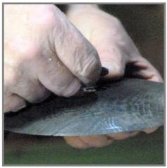
Finally, a small round mirror was glued into the recess in the underside, so completely obscuring the screw chuck hole. Mark advised against using CA glue for fixing the CD/DVD as there can be a reaction with the polycarbonate which results in a white deposit forming (see footnote on next page).
