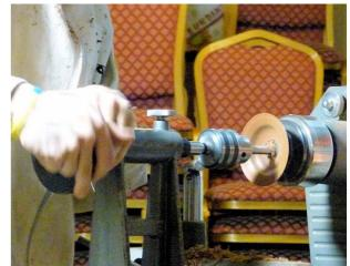
are assembled as a pedestal bowl. The cut was angled slightly inwards to ensure the bowl would sit flat. He then sanded a 45° angle on the opening of the previously drilled hole, as before, and, by inverting the "Unichaser" proceeded to cut the female thread, moving the "Unichaser" in a circular motion, bringing it round to parallel as the thread forms. He kept trying the inner
