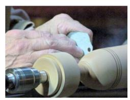
As much as possible of the shaping of the knob/finial was carried out with the tailstock support still present (overhead camera screen shots).
