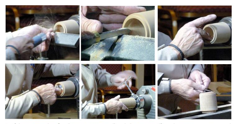
tip of the gouge. A short flute (i.e. a worn out gouge!) works best as it is stiffer and a more aggressive cut can be achieved by using more of the wing of the tool.
