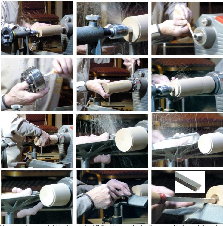
Using the tool-rest as a height guide, a twist drill fitted in a wooden handle was used to bore a hole to the required depth of the box. The box was then hollowed and Steve demonstrated two techniques, firstly using a box scraper (this has the sides bevelled slightly). The use of a spindle gouge was also demonstrated, the technique being to use cuts starting from the centre with the flute at about 10 o'clock and using a scooping action, cutting using the lower
