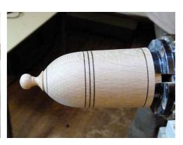
Now to the interesting part texturing and colouring! Steve decided to partly texture the piece so marked out the areas to be decorated in pencil. The texturing was carried out using a Dremel and flexible shaft and a piercing bit, using a light "stroking" motion along the grain until the marked areas had been filled in.
