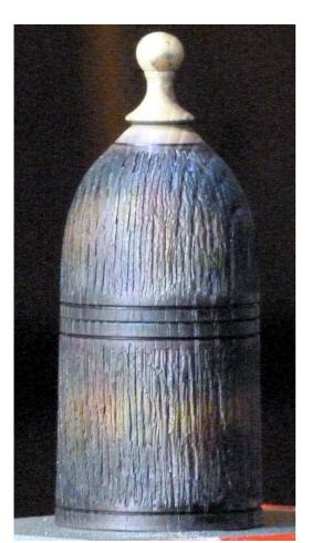
Normally the box would be remounted on a jam chuck for finishing the
