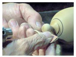
The lid was then removed and the fit slightly loosened, still keeping the barrel shape on the spigot. Steve explained that the fit would change over the next few days but could be adjusted by careful light sanding, assisted by the barrel shape.
