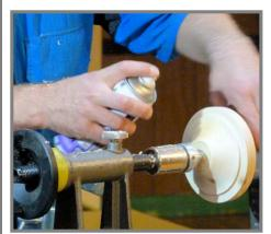
Using the template, the positions of the key features were marked on the edge and face of the work and shaping commenced. The first stage was to create a reduced diameter to the depth of the half bead, and then the large cove was
