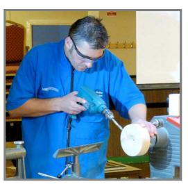
any grain features need to be selected to be appropriately positioned. In this case there were some small knots so the hole was drilled near to these. A lip and spur drill was used in a pistol drill and the piece was rotated to allow a comfortable angle towards the drillina centre of the piece. It is important that the hole is drilled parallel to the base (or slightly 'upwards"). The initial contact
