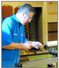
twist drill mounted in a tool handle. He advises a smooth handle in case the drill should jamb in the hole. A small dimple was formed to help with starting the drill, which was then pushed by hand, withdrawing about every 20mm to clear the chips. The drill was long enough to go a little more than half way though the piece.
