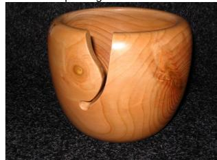
resting on a compound curved surface (not ideal) and I would only get one crack at it I decided to cut the slot first and then drill the hole as I couldn't be sure if the slot would end up in the centre of the hole. I was able to widen the slot slightly using the coarse set of the teeth. I was aware that the slot needed to be smooth so as not to snag on the wool so it needed to be just wide enough to be able to insert double abrasive cloth.
