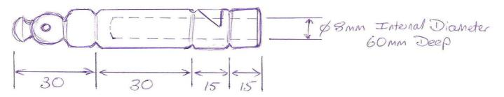
Working between centres Dawn roughed the piece to the round and then drilled an 8mm hole about 60mm deep (using her keyless chuck, newly acquired from Chronos Engineering <u>http://www.chronos.ltd.uk/</u>). Making the hole larger, or deeper gives the finished whistle a lower tone.
