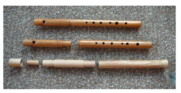
One The advantage of the 4 piece design is that if a part is damaged a replacement can be made. Also the flute can be made on a smaller lathe without the need for specialised long hole drilling equipment. This is a design for a simple fipple flute that Dawn used for dimensions in her demonstration:-
