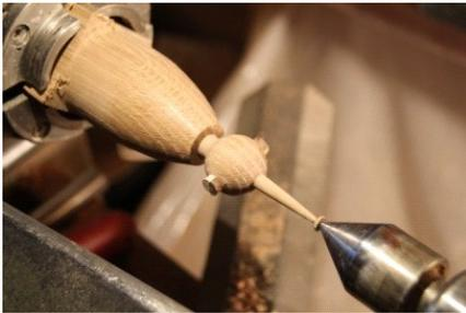
Glue the eyes in place and allow to dry before remounting the oak in the lathe.
