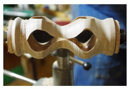
The part turned project showing the developed shape of the central section.
