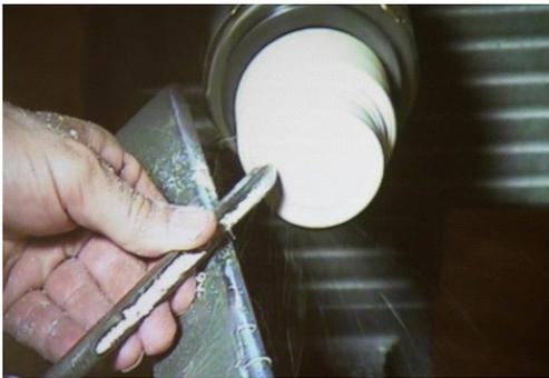
Shaping of the back of the head and refinement of the overall shape continued until such time as the back was finally parted through.
