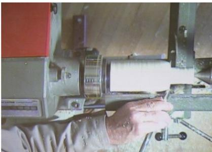
Ted mounted a piece of sycamore approximately 200mm x 70mm x 70mm between centres - which is long enough to produce the head and then later the ears. He reduced this to a cylinder with spindle roughing gouge and long grind spindle gouge and created a chucking spigot.
