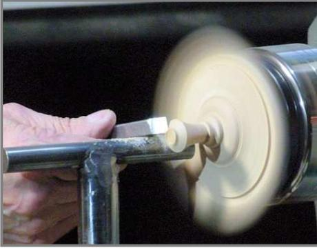
With very light tailstock support, a knob was created using a spindle gouge and skew, final very light cuts being taken with the tailstock removed.
