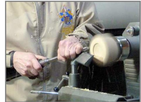
When sanding an "intermittent face", such as the on a winged bowl, it can be useful to make a sanding pad using wood shavings inside a roll of abrasive (rather like rolling a cigarette). This will provide a bit of rigidity to avoid rounding over the edges. It is important not to let all of the abrasive move to the wings of the piece where it is unsupported, or it will grab.
