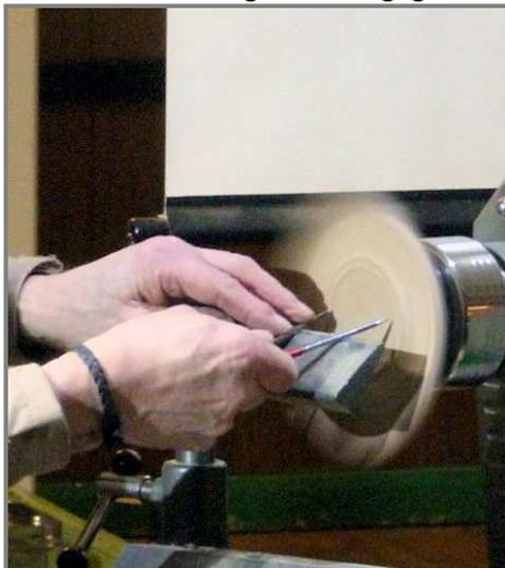
After final refinement of the shape with bowl and spindle gouges, the piece was then hand
