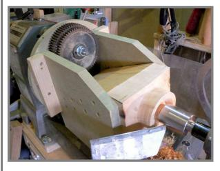
The face was trued up and a 1" hole bored about 1 1/4" deep with a Forstner bit. This would enable me to flare the opening whilst still using the tail centre for support.
