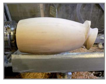
For the hollowing process I decided to use my home made steady. Although the hole already made in the top was about 1 1/4" diameter it was offset to the true axis and I felt that the risk of my hollowing tool rubbing on this eccentric bore might increase the risk of a catch. The steady would reduce the risk of this damaging the piece. note that the angle of flare inside the opening dictates the
