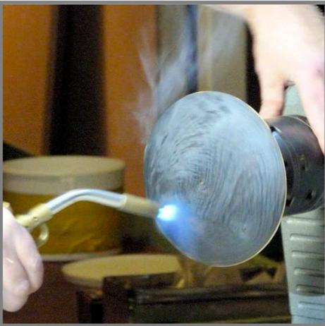
With the wood mounted on a screw chuck, Mark trued and faced it and proceeded to form a smooth curve to a very thin edge. A hand held cabinet scraper, used negative rake at 45° to the surface, was then used to give a fine finish. Then, using a gas blow torch, he scorched the surface. Mark explained that he uses a “professional” torch that runs MAPP gas. This burns at a much higher
