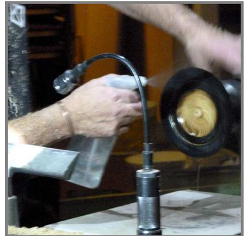
embers should cause an explosion. It is also important to make sure the lathe is clear of shavings and dust when performing the scorching. Mark laid a fire proof board on the lathe bed for added protection.
