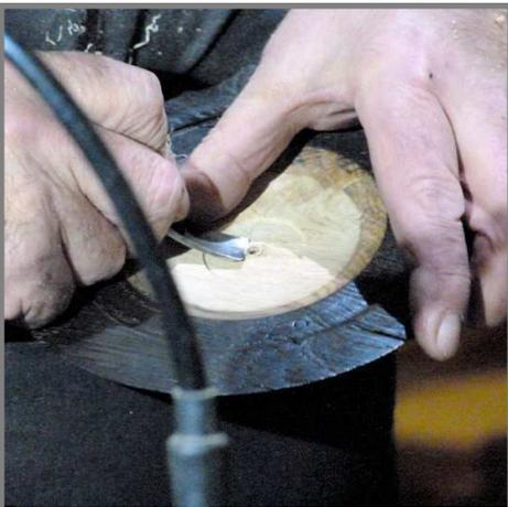
The piece was then reversed on the screw chuck for facing and hollowing. Much careful measuring with a vernier caliper ensued while the piece was hollowed to form a shallow bowl with a recess at the rim and another small recess in the bottom (again, the reasons for these would become clear later!). Great care was needed to turn as much of the centre away as possible without hitting the screw chuck.
