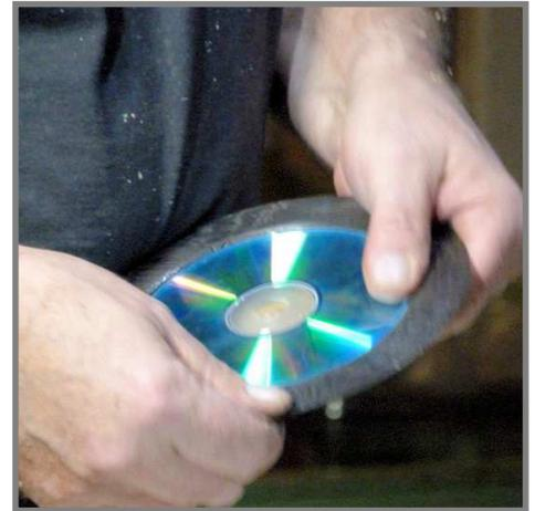
Finally, a small round mirror was glued into the recess in the underside, so completely obscuring the screw chuck hole. Mark advised against using CA glue for fixing the CD/DVD as there can be a reaction with the polycarbonate which results in a white deposit forming (see footnote on next page).
