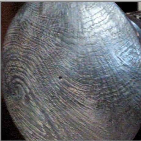
temperature than butane or propane and so scorches much more quickly, hence reducing the stress to the wood which can result in surface cracking. The downside is the cost (£50 or so for the torch head and £15 or so for the gas) but the process is so quick that little gas is used. The bonus is that the torch burns hot enough to use for brazing steel together. After scorching, the piece was sprayed with water to cool it and then
