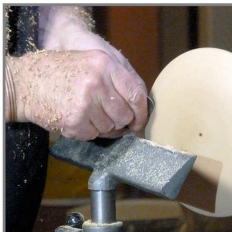
During the evening, Mark used only two turning tools; a small bowl gouge and a shear scraper, and did no sanding at all.
