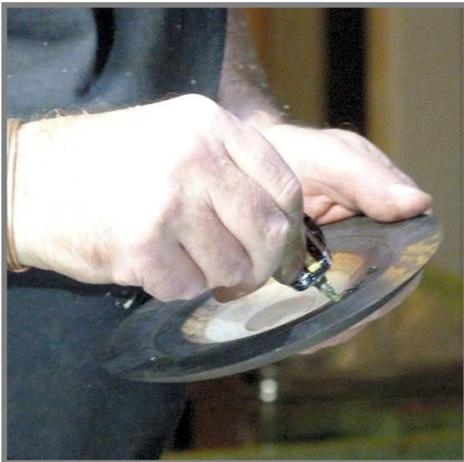
Using CA glue, a pre-turned oak disk was fixed into the small internal recess to cover the screw chuck hole. Then, using impact adhesive, a CD was fixed (“tracks” facing up) into the top of the bowl. This made a nice contrast with the scorched oak (CDs and DVDs often display differing hues).
