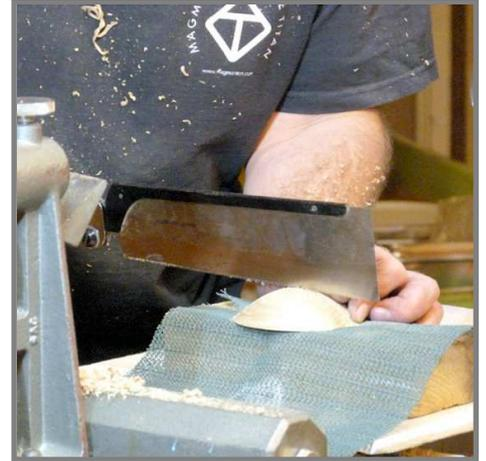
The final item was a “vase”, again turned from a small piece of oak. After turning a shallow bowl, Mark cut this in half (along the grain) and joined glued the two halves together. A small flat was formed by sawing off a small section to allow the vase to stand up. Finishing of the open face is optional and Mark showed several alternative styles that he has used.
