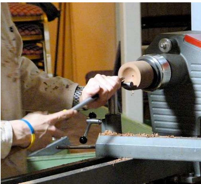
Then, with the piece mounted in the chuck Adam hollowed out the bowl recess and shaped the outside using a bowl gouge, producing in effect a large egg cup. This was sanded and finished with cellulose sanding sealer and then friction polish.
