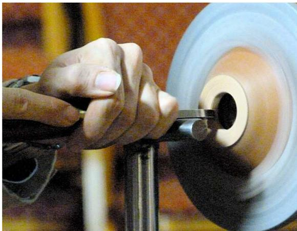
gouge to produce a face for the base to sit against when the two parts are assembled as a pedestal bowl. The cut was angled slightly inwards to ensure the bowl would sit flat. He then sanded a 45° angle on the opening of the previously drilled hole, as before, and, by inverting the "Unichaser" proceeded to cut the female thread, moving the "Unichaser" in a circular motion, bringing it round to parallel as the thread forms. He kept trying the inner
