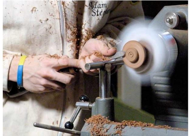
Now Adam demonstrated the use of the Ashley Isles "Unichaser" thread cutting tool. This single tool can cut both the male and female threads by simply turning the tool over.
