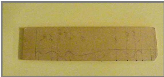
A template was used as before to mark the positions of the key features. Using a vernier calliper (with rounded off points) the piece was "blocked out" using the beading and parting tool. Richard commented that
