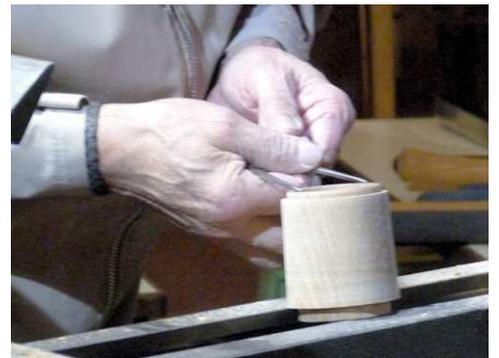
tip of the gouge. A short flute (i.e. a worn out gouge!) works best as it is stiffer and a more aggressive cut can be achieved by using more of the wing of the tool.
