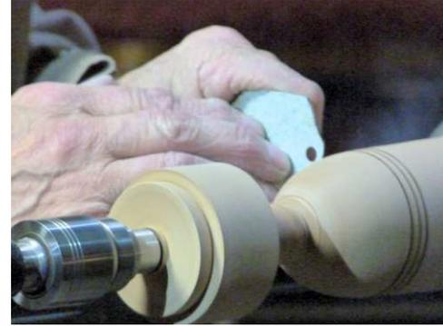
As much as possible of the shaping of the knob/finial was carried out with the tailstock support still present (overhead camera screen shots).
