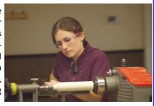
Emma has adapted her turning technique to overcome the limitations of her height, not only raising her elbows and even standing on tiptoe, but grinding her tools to facilitate access to the wood. For example, she uses a large spindle roughing gouge which has a bevel close to  $90^{\circ}$ .
